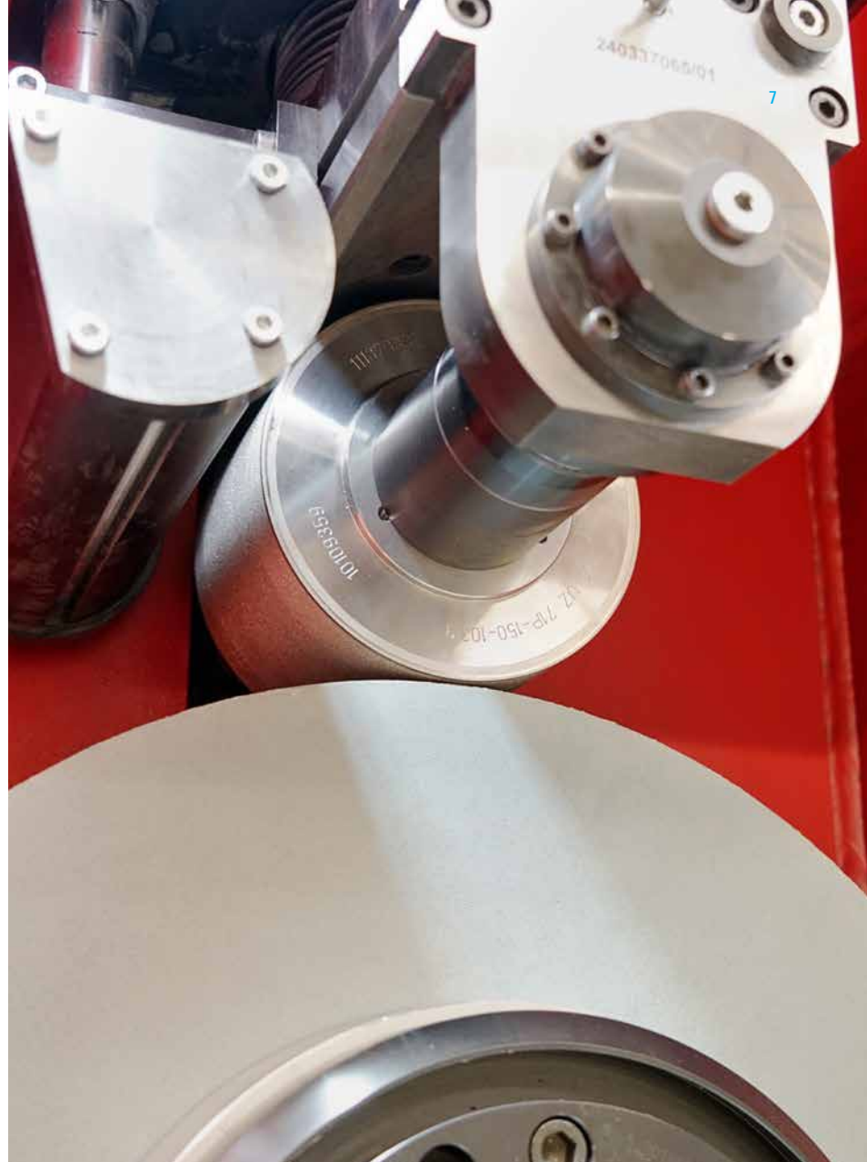
▲ Overhead dressing system PEA-K for IPD and CD grinding methods designed for a grinding wheel width of up to 200 mm.
