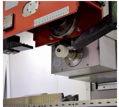
Additional horizontal grinding spindle , 18,000 rpm; 13 kW
