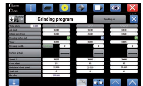
3 layer automatic grinding cycle: roughing, semi-finishing, finishing, spark-out with integrated dressing cycles. Only a few parameters are required to complete the cycle.
